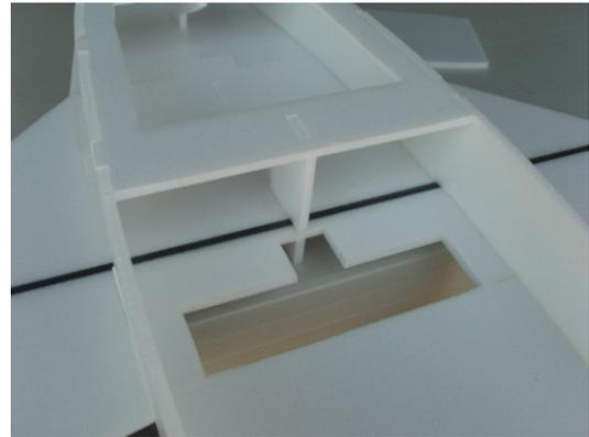
7. Vertical Tail. Next get the two vertical tail pieces. Fit them into the remaining slots with the tabs on the tail pieces.
