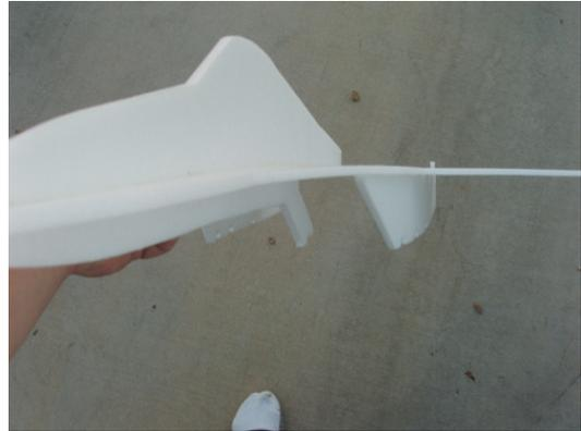
5. Bottom Fuse. Find the bottom fuse piece to enclose off the bottom. Glue into place.
