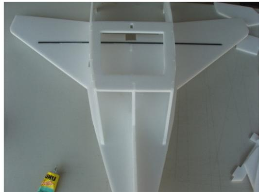
6. Rear Fuselage. Flip your plane over so it's sitting right side up. Find the rear fuselage piece and attach. **NOTE: You can go ahead and mount your motor now, if you complete Step 8 first. It might be easier for you, but not necessary. See step 10 for details.** You will note that there are tabs that fit into the slots.
