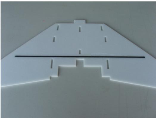
2. Front fuselage assembly. Next, we recommend using epoxy for this step too, it makes the rest of the assembly go a little quicker if you have a nice rigid
