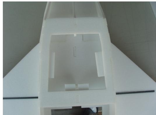
8. Reinforcement Piece. This is the little rectangle piece that is left. It goes under the plane to reinforce the box you created. We recommend using epoxy on this piece. It is mounted near the motor area.
