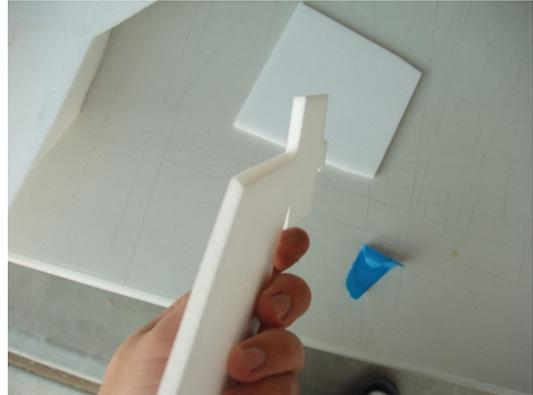
Here (below) you can see the beveled gap in the aileron to allow for free movement positioned on the bottom of the plane.
